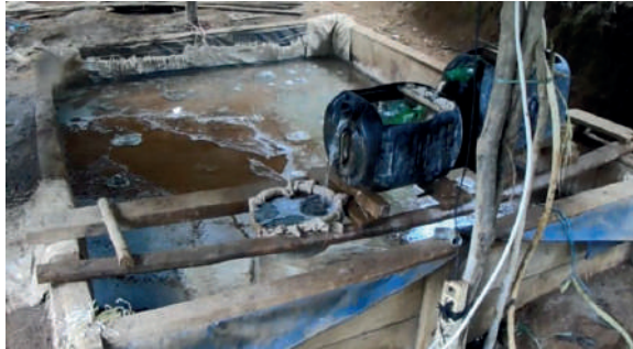
Photo 3.5 Cyanidation Process Using Zinc Ash
