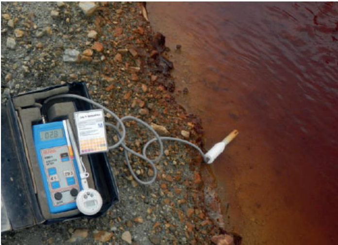
Photo. 5.4 pH Measurement with pH Paper and pH Meter
