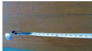
b The tape measurement is pulled tight until it binds the reference nail
