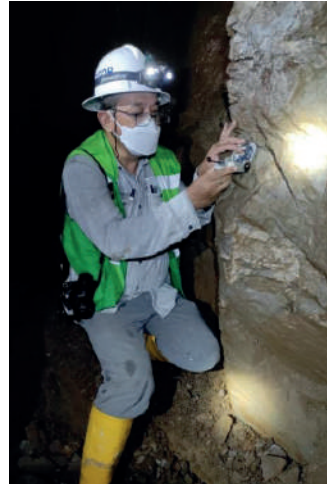
b) Strike and dip measurement
