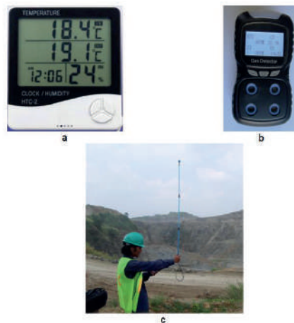
Figure 4.16 a) Simple Temperature and Humidity Measuring Tool (Tokopedia) b) H 2 S, CO, O 2 Detector and Exploding Gas c) Wind Speed Measuring Tool
