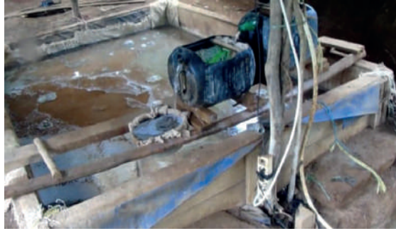
Photo 4.21 The Immersion Method using Zinc Powder
