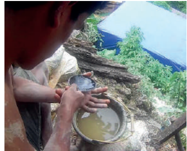
Photo 2.5 a) Gold Vein Sampling b) Gold Content Checking
