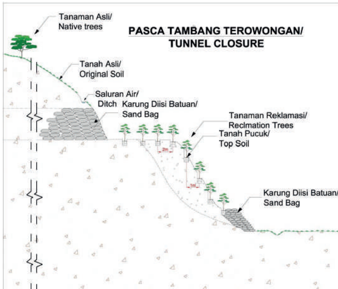
Figure 5.4 Post-Mining Illustration Around the Tunnel
